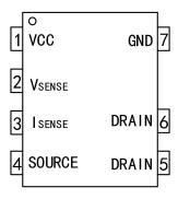
Figure 2.1: G5238MK Series (7 Lead SOP7 Package)
