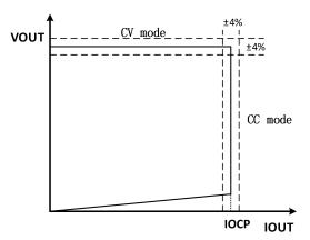
Fig.1. Typical CC/CV Curve
