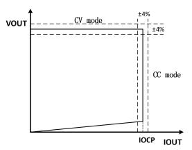
Fig.1. Typical CC/CV Curve
