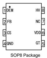
Fig.1. G1602C Pin Configuration
