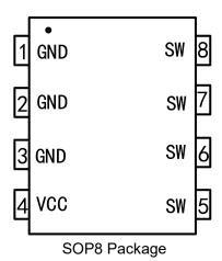
Fig.1. IW7700A Pin Configuration
