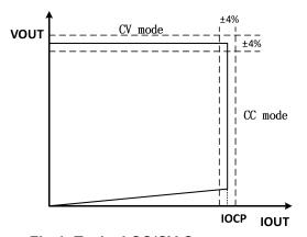
Fig.1. Typical CC/CV Curve
